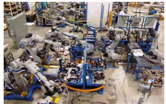
Automated turnkey resistance welding system during pre-shipment testing and acceptance trials
