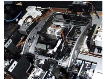
Our fixture assemblies feature robust design and construction, copper pneumatic lines, spatter shielding and special coatings to prevent weld contaminant build-up.
