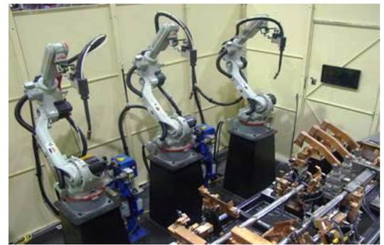
MIG welding system including complex fixturing and “ferris wheel” material handling system
