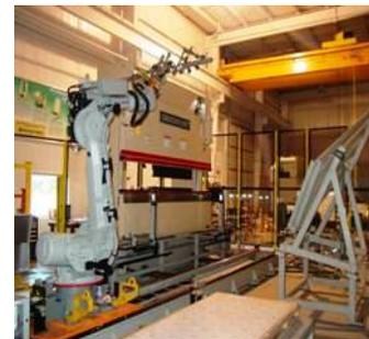
Stacking / palletizing robots increase throughput by manipulating large parts off of conveyor lines (left) or while performing bends in a press brake (right).
