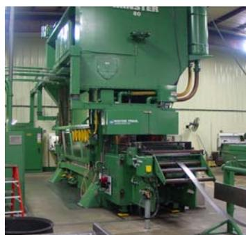
Three axis ‘through the window’ transfer mounted on a 144” bed press
