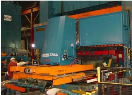
Blank loader with automatic centering station assures proper blank loading position, critical to the first operation draw. This servo module is outfitted with a 'compound sled' to extend reach of load and unload stroke.
