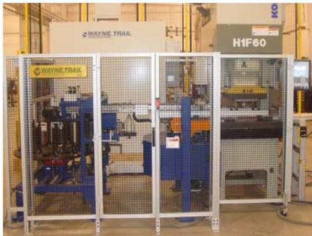
Gap frame press automation with automated blank destacking system
