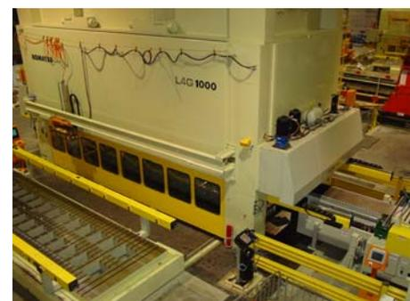
Three axis ‘through the window’ transfer mounted on a 295” bed press
