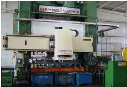
Two module transfer with lateral die access in the run position
