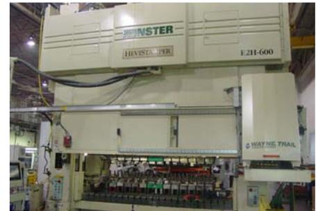
Two module transfer with lateral die access in park position
