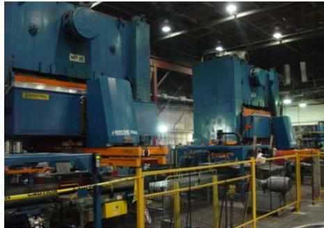
Loaders/unloaders utilize a simple, robust mounting bracket to simplify field mounting in retro-fit applications. Purpose built 'rotate and load' unit is used to move product in and out of special forming station located between presses.
