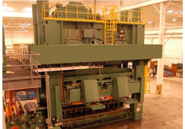
4 Module - 3 Axis Servo transfer mounted on a 240" x 108" press
