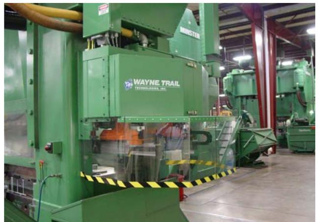
3 Axis "through the window" Servo transfer mounted on a 144" x 48" press
