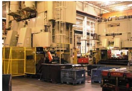
Four module transfer with vertical die access in park position
