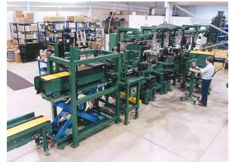
Dedicated Tube Manufacturing systems often require custom made tube hoppers. This system utilizes a scissors lift to elevate skids of square tubing, allowing the tubing to be automatically fed in the bending and forming stations.
