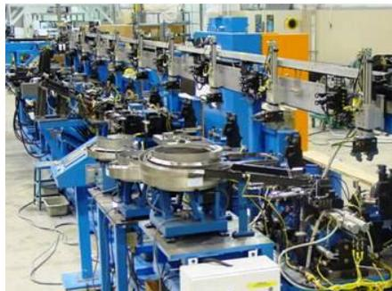
Feeder Bowls are often used in tube manufacturing systems to feed parts required to assemble various post bend components.
