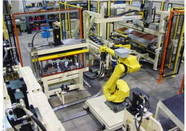
Flexbending® system robotically loading of bent tubes into a 200 ton press
