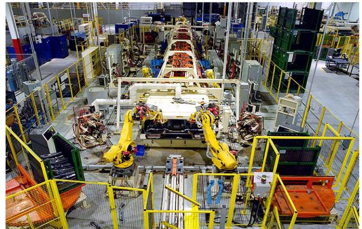
Total system design can be provided, accurately locating all line components. Master line control provides a central point for monitoring of all system modules. Interlocked barrier guards provide for operator safety. Scrap is directed into a central conveying system and removed outside the system guarding. Hydroform fluids are contained within the system for cleanliness and safety. Full installation service is available to rig, wire and start-up your complete system.
