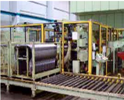
High performance part transfers are supplied for all automated pre- and post-hydroform systems. Transfers and lift units can be servo, hydraulic or pneumatically driven – depending on through-put and application requirements. Tooling is customized for each process module within the system.
